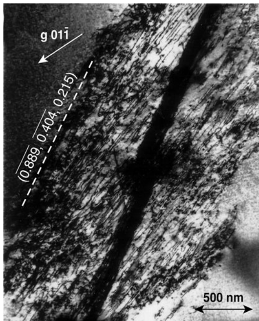
Fig. 2 Large array of dislocation loops in the cubic austenite phase of the \text{Ni}_{50.5}\text{Ti}_{49.5} specimens after one thermal cycle that was imaged near [111]_{\text{A}} with \mathbf{g} \ 01\bar{1} . Under these imaging conditions, the dislocation line directions, \mathbf{u} , are parallel to [020]_{\text{A}} and are perpendicular to the foil surface; hence the dislocations have a screw character. The strong-contrast dislocation band through the array is composed of mixed orientations and is parallel to (0.889, 0.404, 0.215) , according to Ref 5
